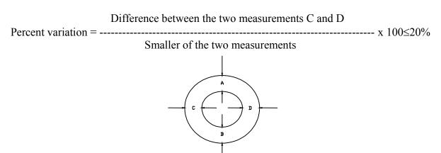
This calculation shall be repeated for dimensions A and B.
